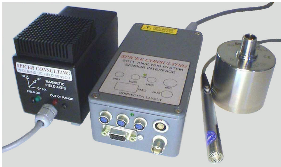
Left to right: SC20 wideband DC sensor, SC11 Sensor Interface, B&K 4190 microphone, Wilcoxon 731A accelerometer
